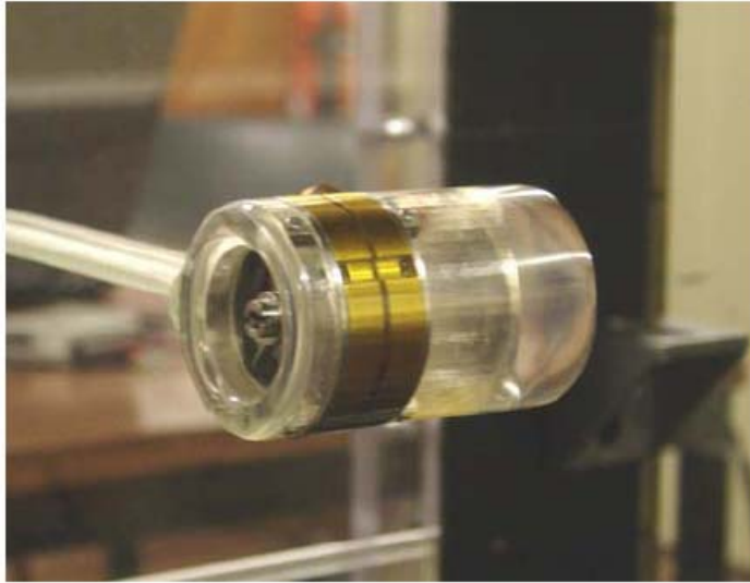
Figure 2. Prototype turbine installed in the experimental section of an 18" \times 18" wind tunnel.
